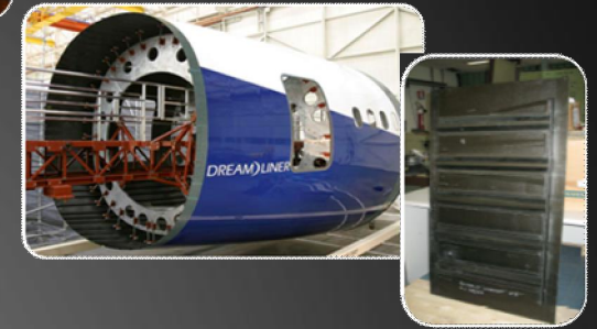
ARCA – composite panel with improved vibro-acoustic properties and weight reduction
