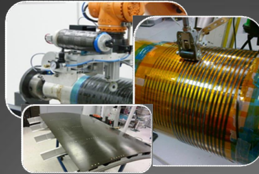
TECOP – Thermoplastic composite fuselage components (manufacturing optimization)
