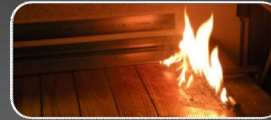
Green Regional Aircraft – Analysis of fire performance of composite components
