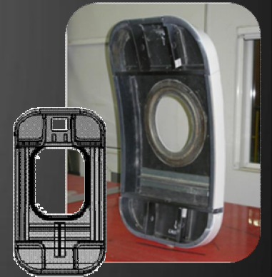
CESPERT – Thermoplastic composite emergency door with hail impact resistance and weight reduction
